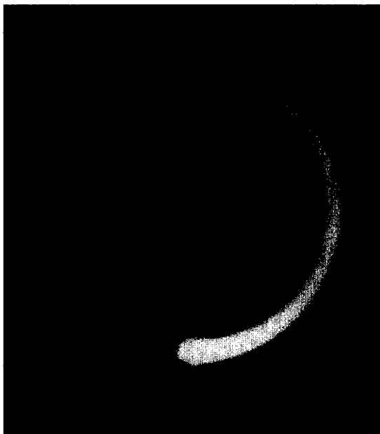
Fig. 2. Photograph showing the luminescence decay of a solid phosphor on a rotating disc.
